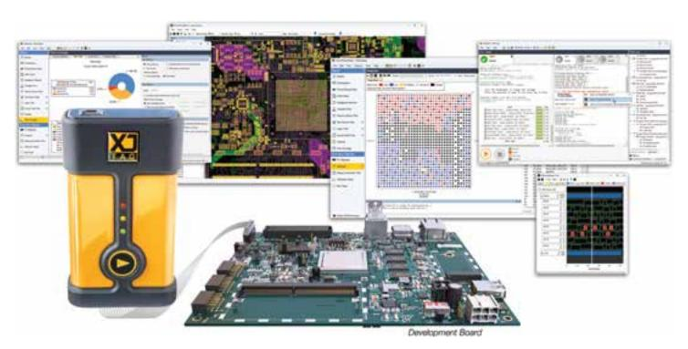
Boundary scan controls devices from the inside, via a simple 4-signal interface to the board. It is particularly useful for device packages such as Ball Grid Array (BGA), where the individual balls are inaccessible to conventional probes.
