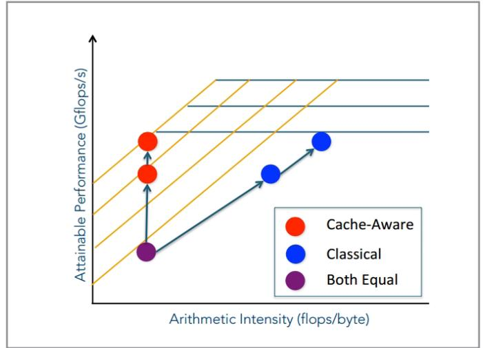
Figure 2. How a point moves in classic versus cache-aware roofline model
