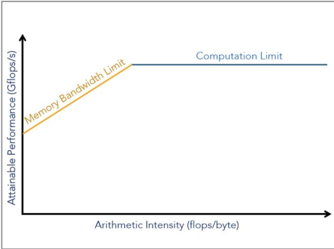
Figure 1. Roofline visual performance model
