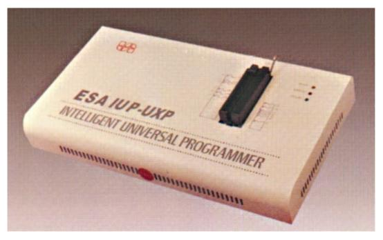
**ESA IUP-UXP** is an advanced version of our earlier model ESA IUP-XP, which works through a PC's parallel port & USB port. It features a 48 pin universal pin driver and an expandable TTL pin driver. It supports over 7000 devices including PAL, GAL, CEPAL, EPLD, PEEL, MAX, MACH, PLSI, EPROM, MPU/MCU etc. ESA IUP-UXP works in various operating systems, Windows 9x/NT/2000 and XP.
