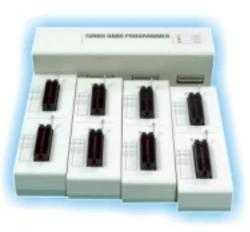
The ESA GP8-XP is a gang programmer, which works through the PC's USB port or parallel port. It features 8 fully isolated 48-pin ZIF sockets, extremely high throughput, standard 5V and 3V chip support, device insertion and continuity check. With PC-based design and device update through software provides flexible and quick access to the new chip support. ESA GP8-XP supports EPROM, EEPROM, FLASH in the introduction. Future software update will include 87C5x, 89C5x, and PIC16Cxx microprocessor.
