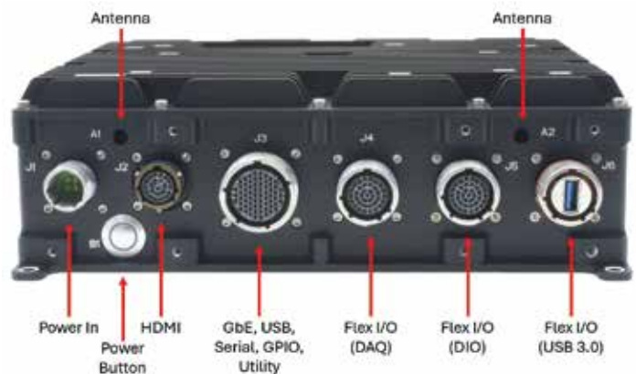
SabreCom-JSP Rugged computer with maximum configuration flexibility
