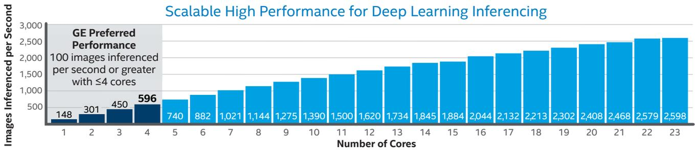
**Figure 2.** The Intel® Xeon® processor E5-2650 exceeded GE’s inferencing performance target by nearly six times on four cores, and demonstrated steady, scalable performance for solutions needing more cores.
