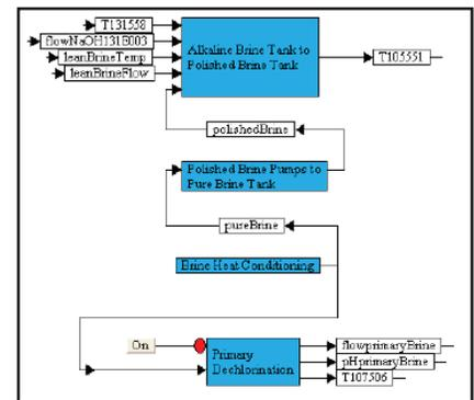
Embed SE model of plant training simulator. The top three blue compound blocks represent the purification and temperature control of the brine prior to electrolysis. During this process, heat is exchanged with other hot streams that have already passed through the electrolyzers. The bottom blue compound block treats the spent brine to remove dissolved chlorine.
