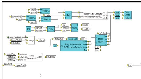
Subsystem 1 of two sensorless PMSM motors using sliding mode observer estimation of rotor position. Sample rate is 10 kHz running both motors on a Piccolo F28036 with 50% utilization.
