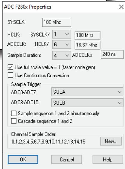
Embed model of a 400 kHz digital buck voltage converter that uses a built-in optimizer to tune the PI control against the simulated buck circuit (left). Once the controller gains are tuned, the embedded control is created with ADC input synchronized to the PWM output, along with background tasks to monitor temperature and set status LED bank (below, left). Embed auto-code generation creates the C file used to implement the control on the target (below).
