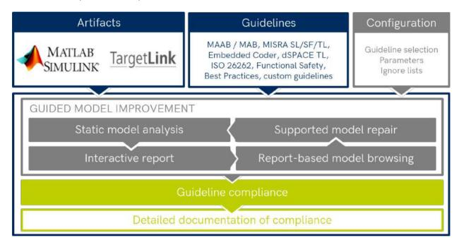
MES Model Examiner® analyzes software models for guideline compliance and guides the user through the repair and improvement process.
