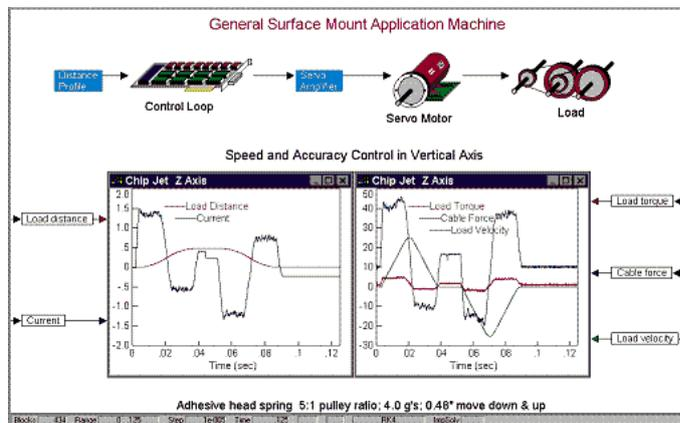
Embed GSM1 model. Current, Load Distance, Torque, Velocity and Cable Profiles
