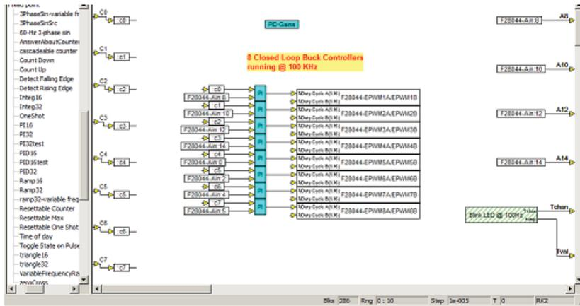
Embed source diagram to control TI DC-DC 8-Buck Converter Kit
