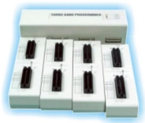
The ESA GP8-XP is a gang programmer, which works through the PC's USB port or parallel port. It features 8 fully isolated 48-pin ZIF sockets, extremely high throughput, standard 5V and 3V chip support, device insertion and continuity check. With PC-based design and device update through software provides flexible and quick access to the new chip support. ESA GP8-XP supports EPROM, EEPROM, FLASH in the introduction. Future software update will include 87C5x, 89C5x, and PIC16Cxx microprocessor.
